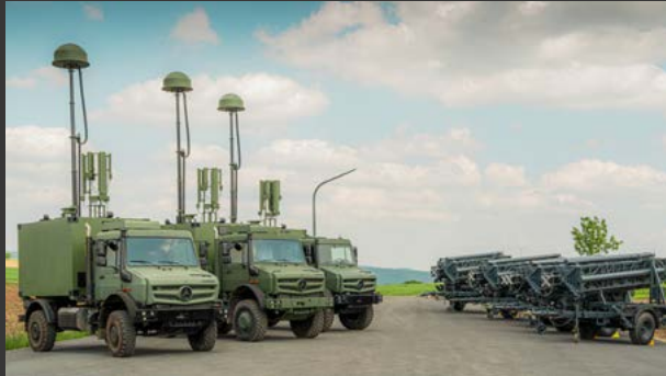
AARTOS™ C-UxS Compact Shelter 4x4 Unimogs and 25 meter masts
