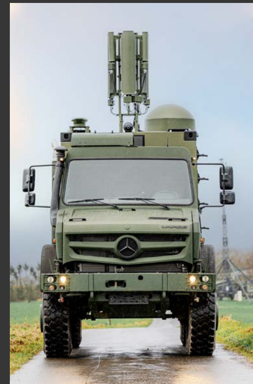
AARTOS™ Unimog equipped with X9 RF drone detection and 360° fixed bands sector jammer
