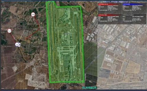
Angle of Arrival drone triangulation combined with drone protocol decoding for reliable airspace security
