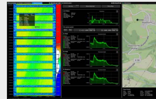
Full-band real-time spectrum analysis including drone protocol decoding
